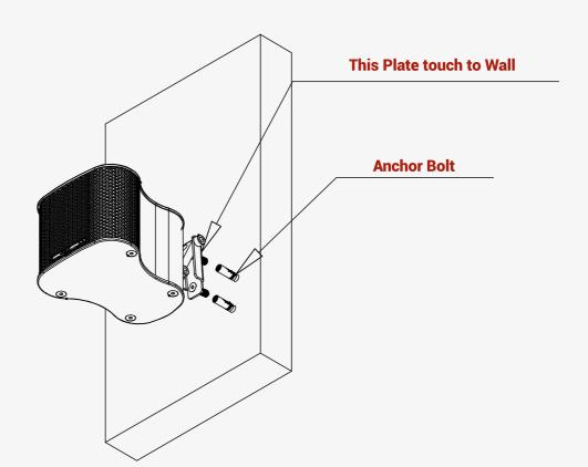
The illustration above displays the wall mounting arrangement for the ST 3 loudspeaker and identifies the essential hardware supplied.
